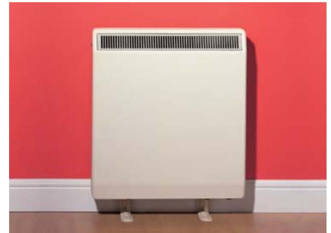
At approximately 11pm an automatic time clock will switch the metering to the low rate, (known as off peak); at this point the heaters are turned on. The heaters will then charge up and store the heat. The actual amount of heat that is stored will depend on how you have set the controls for that heater.
