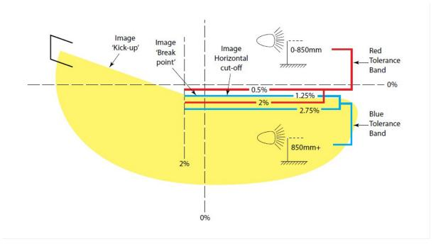
Check on dipped beam and determine that:
